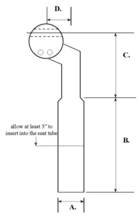
**D.** This measurement needs to be from the center of the lug to the center of the seatpost diameter.
